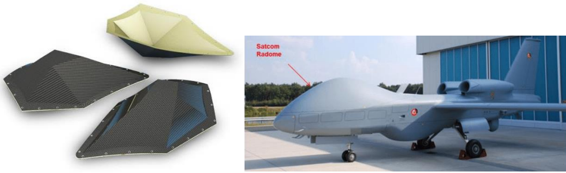
Figure 14-1: Examples of radomes with asymmetries
